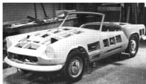
Full-size wooden model, called a 'buck'. This was used to shape body panels on.
